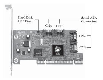
Figure 1. Serial ATA 4-Channel RAID layout
